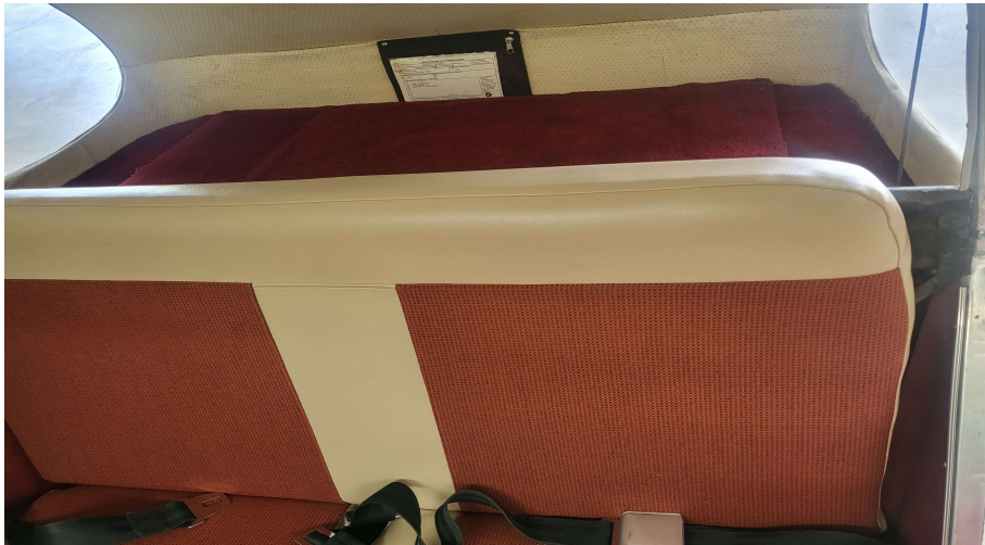
The shelf aft of the crew seat. The lid is access to luggage etc storage
